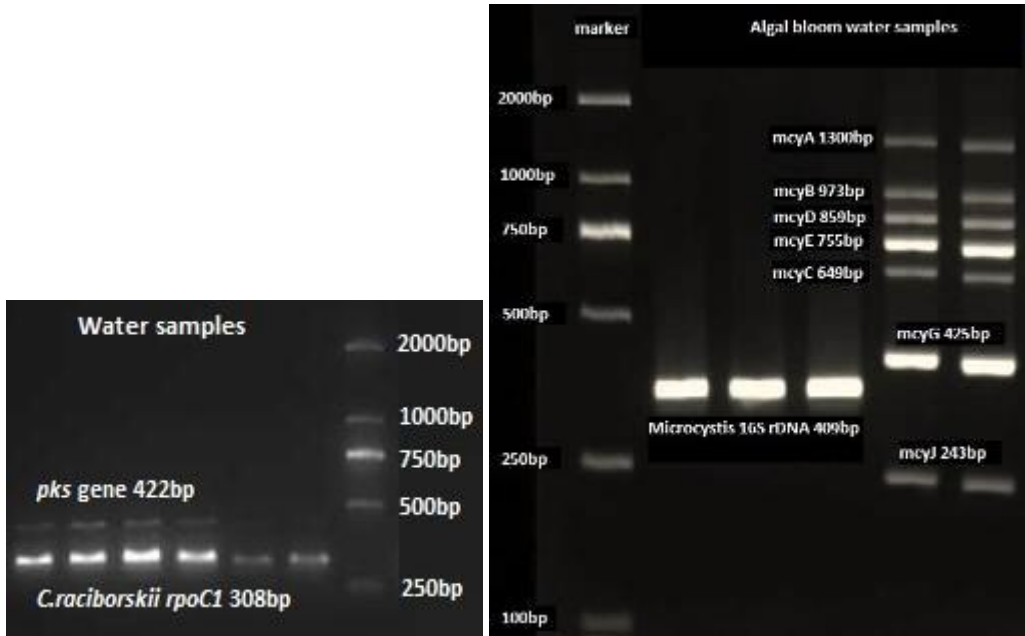
Figure 11. Multiplex PCR results of pks/C. raciborskii rpoC1 and mcyA-J/Microcystis 16S rDNA in water samples.
