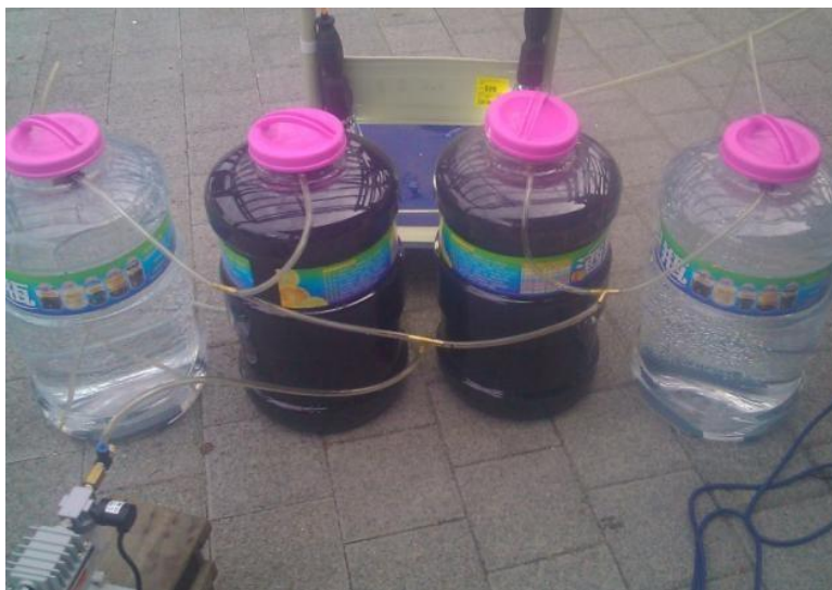
Figure 1. A model of the hydrogen sulfide bioreactor adsorption system.
